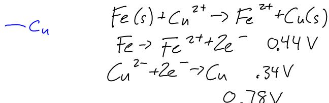
Our observed voltage was .681V while the calculated voltage was .78V
