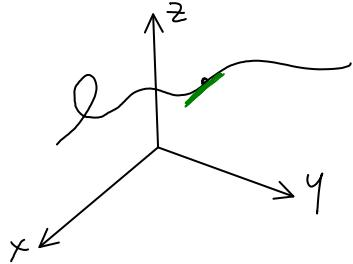
$r'(t)$  gives a vector tangent to the space curve defined by  $r(t)$ . The length of  $r'(t)$  is the speed at which the particle moves.
